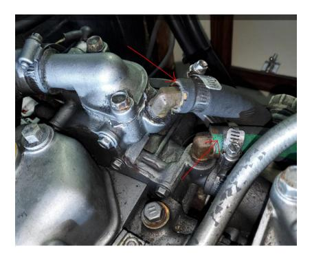
Now let's remove old coolant from the engine by opening the Four tap valves.
